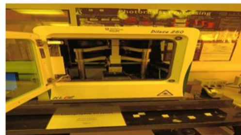
Figure 13. The dilase 250 machine from KLOÉ, a high-precision system used for DLW in photolith
